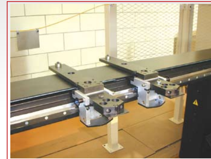
Standard 5-Axis Backgage
