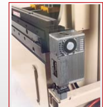
Optional CNC Crownable Filler Block
