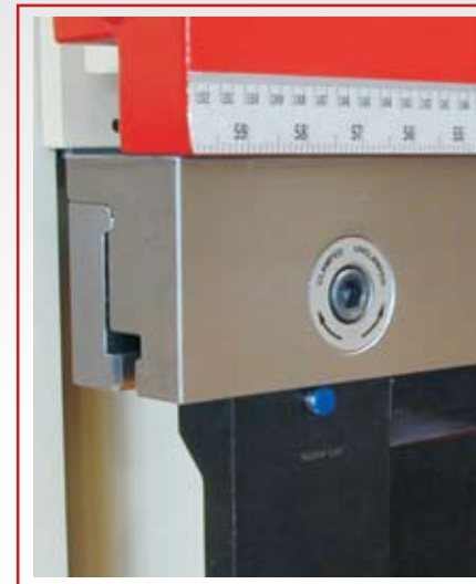
Standard Quick Change Ram Nose
